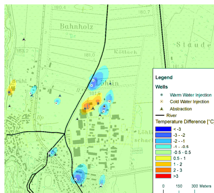
Calculated temperature plumes in the test site Bahlingen with basal and surface heat flow
